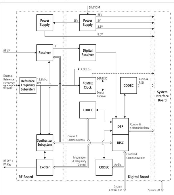
Figure 2.1 Reciter high level block diagram
