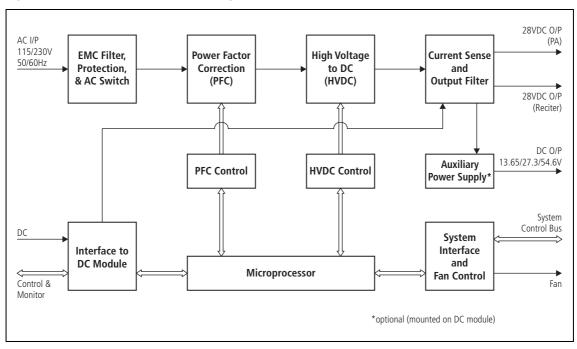
Figure 12.3 PMU AC module block diagram
