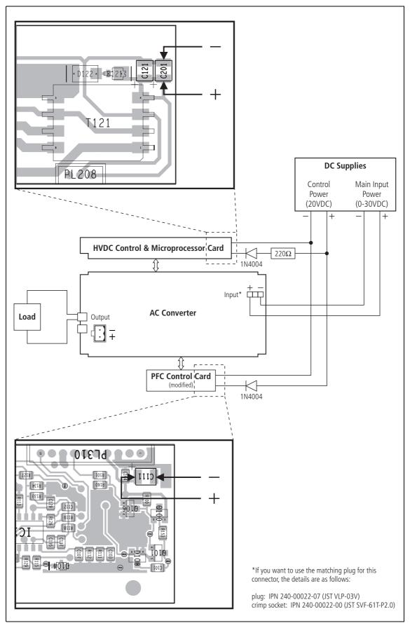
Figure 13.11 AC converter test equipment set-up
