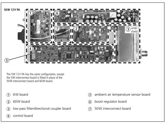
Figure 8.2 Identifying the circuit boards in a 12V PA
