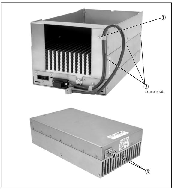
Figure 9.1 Removing the airflow duct and cover
