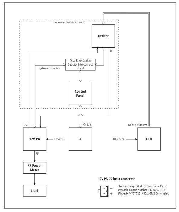
Figure 8.9 Recommended test equipment set-up for circuit board checks - 12V PA
