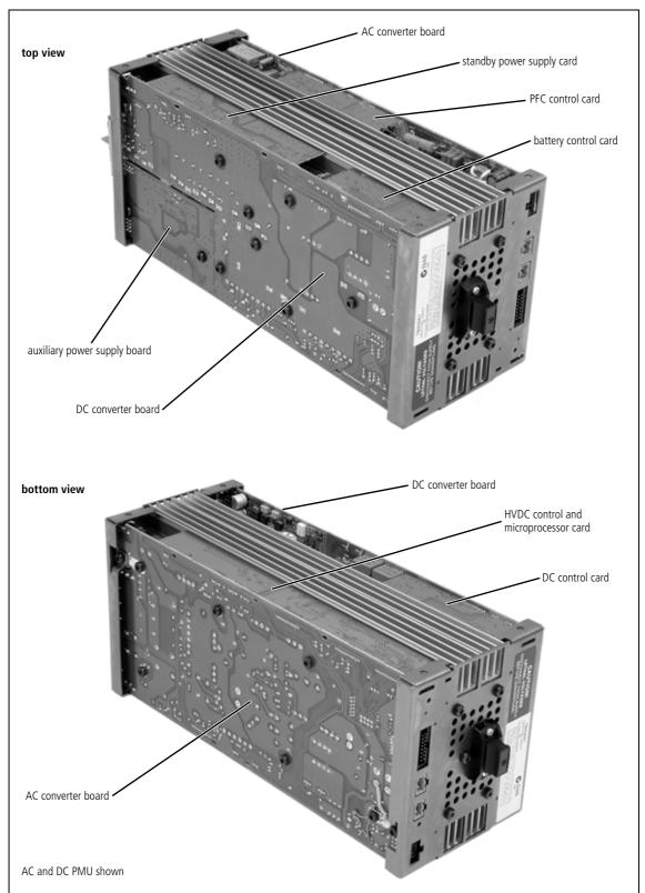
Figure 13.1 Identifying the boards and cards in the PMU
