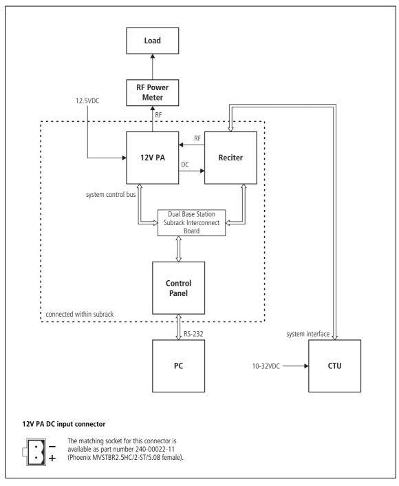
Figure 8.4 Recommended test equipment set-up for initial checks - 12V PA
