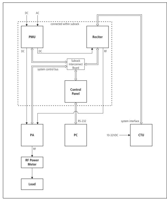
Figure 8.8 Recommended test equipment set-up for circuit board checks - 28V PA
