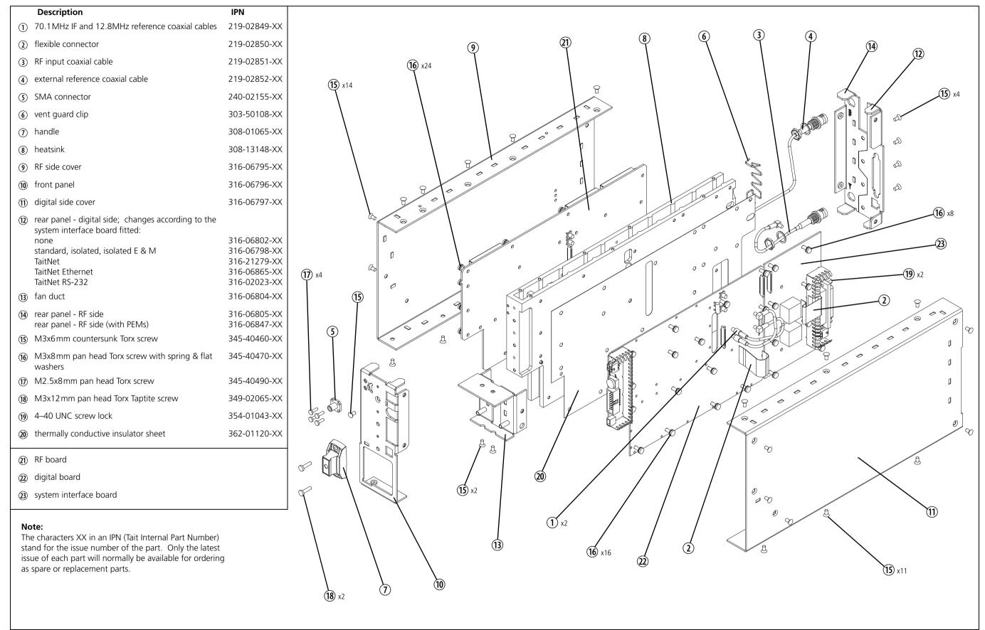
The TB8100 power amplifier (PA) is a modular design with the circuitry divided between separate boards. These boards are assembled onto a heatsink in different configurations in different models.
