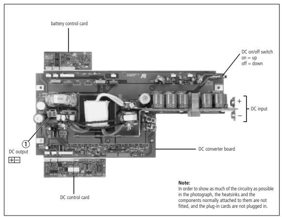
Task 2 — Check Battery Control Card The battery control card monitors the battery voltage and sends the voltage digitally to the microprocessor. When the DC converter is running without a microprocessor, as shown in Figure 13.5, the digital information will have no effect on the operation of the converter. The only analogue circuitry that will be active is the window comparator on the battery control card. This protects the converter from operating on the wrong input voltage.
