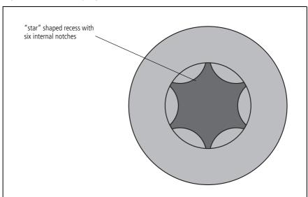
Figure 1.2 Identifying Torx screws
