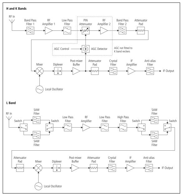
Figure 2.7 Reciter UHF receiver RF circuitry block diagram
