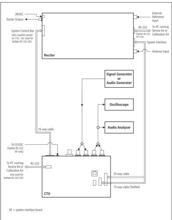
Figure 3.6 Recommended test equipment set-up for audio checks
