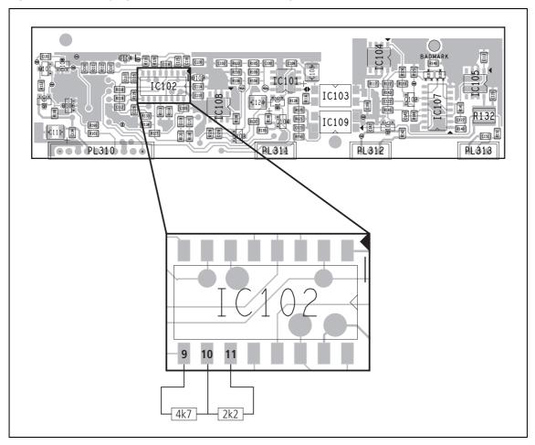
Figure 13.13 Modifying the PFC control card for testing the AC converter
