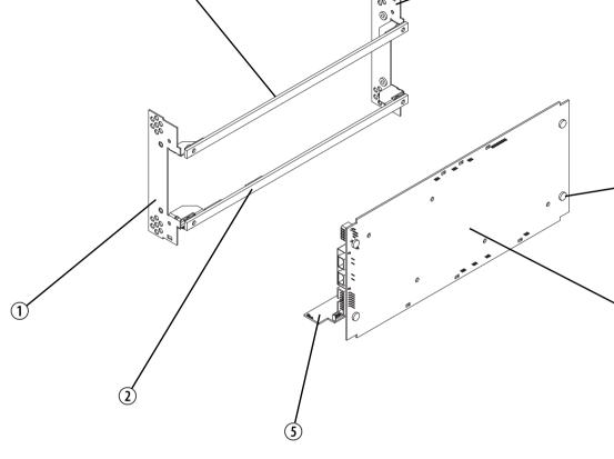
**AC PMU** This drawing shows the blanking plates fitted to the front and rear panels in an AC PMU. These plates cover the holes normally covered by the DC module heatsinks.
