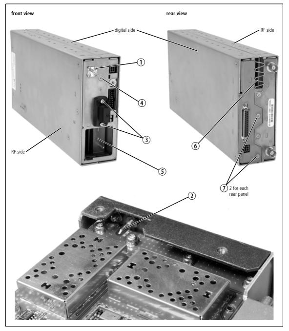
Figure 4.1 Removing the front and rear panels
