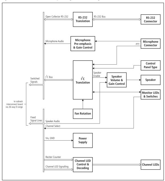
Figure 17.2 Multi-reciter control panel high level block diagram
