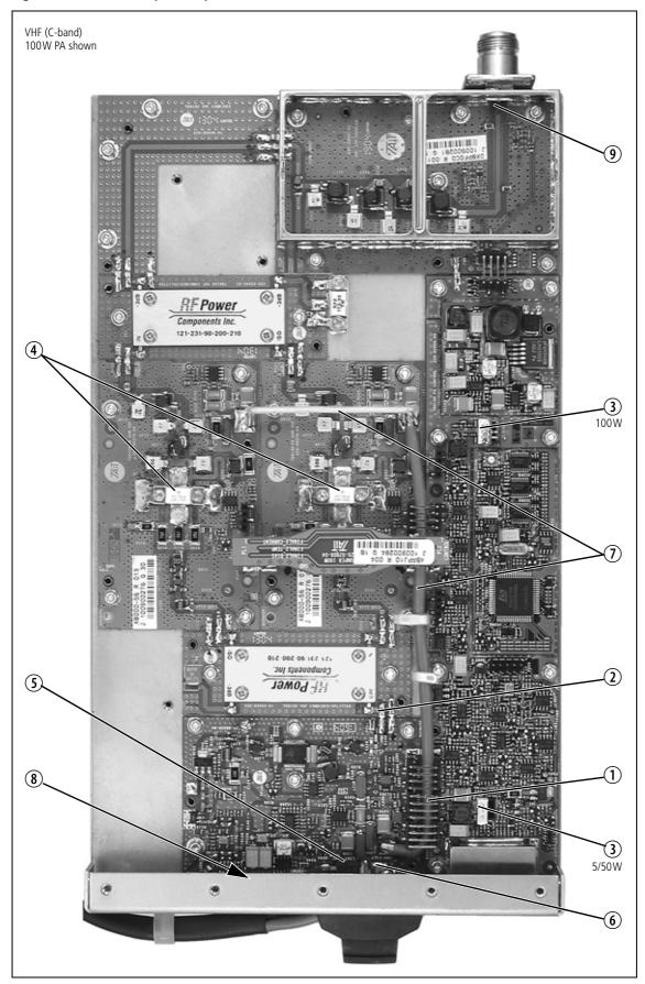
Figure 8.6 Visual inspection points for a 28V PA
