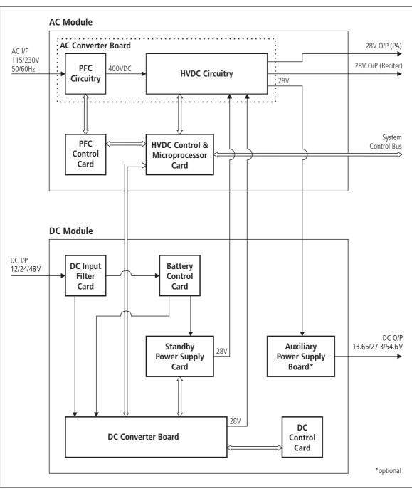
Figure 12.1 PMU high level block diagram
