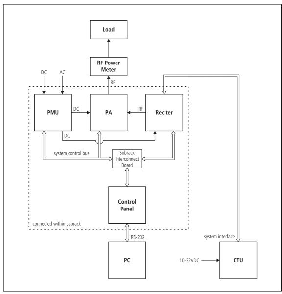
Figure 8.3 Recommended test equipment set-up for initial checks - 28V PA
