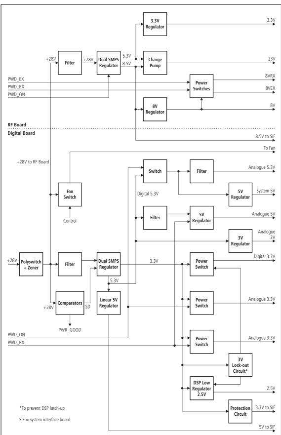
Figure 2.13 Reciter power supply block diagram
