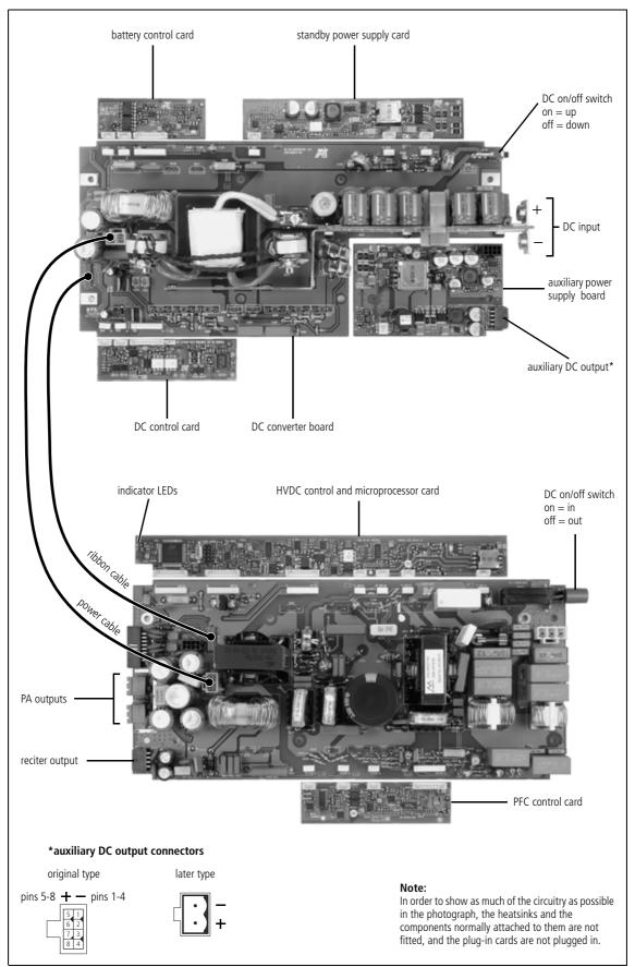
Figure 13.8 Checking the DC converter with microprocessor control
