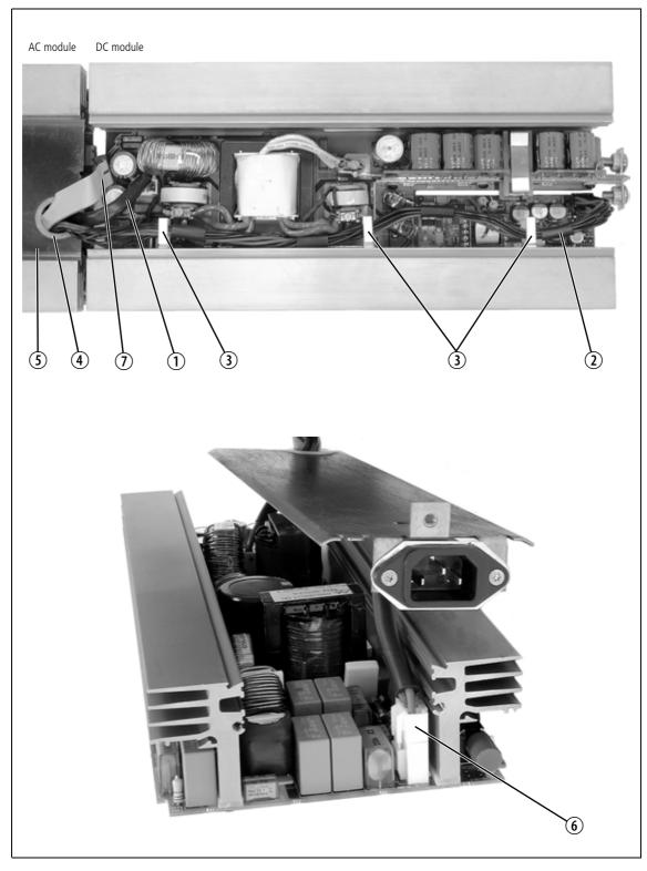
Figure 14.2 Disconnecting the AC and DC modules
