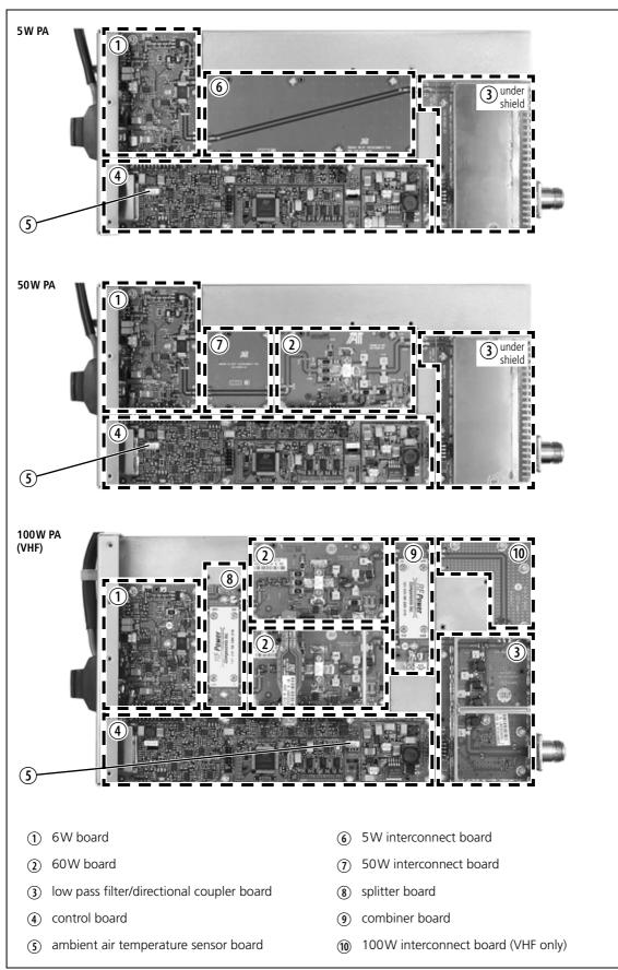
Figure 8.1 Identifying the circuit boards in a 28V PA
