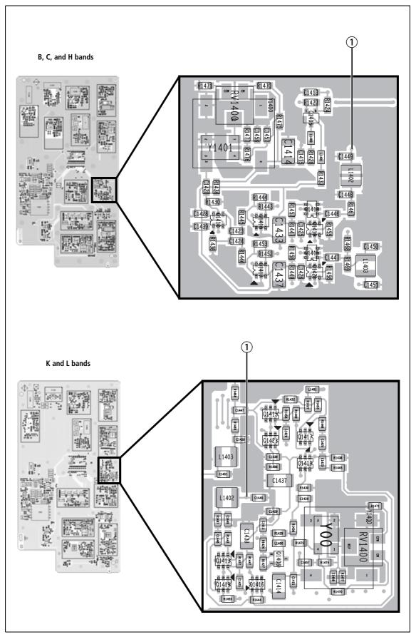
Figure 3.4 Location of the 12.8MHz clock test point on the RF board
