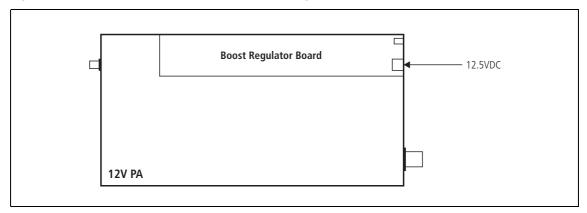
Figure 8.16 Location of test points on the boost regulator board
