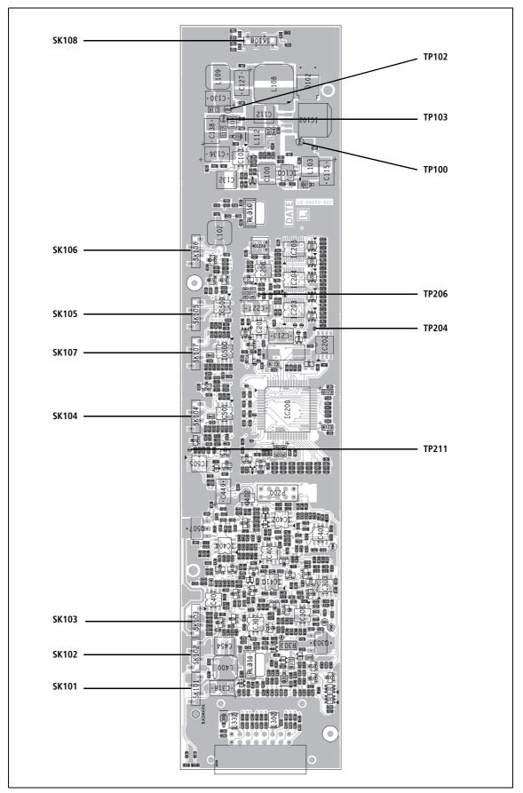
Figure 8.10 Location of test points on the control board
